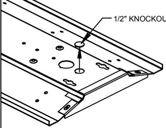
**OPTIONAL-PENDANT MOUNT:** Prior to Step 5, remove 1/2" knockout from both ends of fixture.
