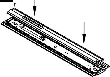
**OPTIONAL-PENDANT MOUNT:** Reinstall the driver cover making sure all wiring is tucked safely under the cover. Test the fixture.
