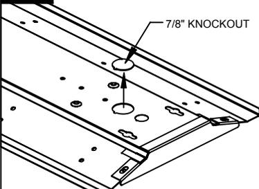
Remove 7/8" knockout from bottom of fixture in desired location to allow for wiring. Bring supply wiring thru and wire in accordance with all national, state and local codes.
