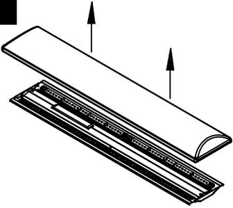
**CAUTION:** EDGES MAY BE SHARP: Carefully remove lens from fixture by gently sliding lens over the edge of the fixture one side at a time, and set aside.
