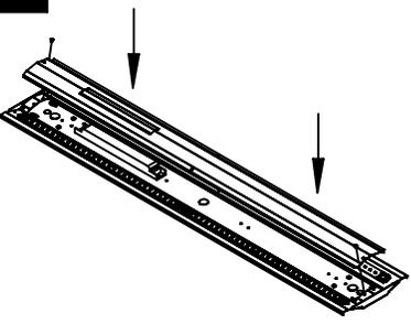
Reinstall the driver cover making sure all wiring is tucked safely under the cover. Test the fixture.
