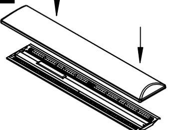
**OPTIONAL-PENDANT MOUNT:** Reinstall the lens by placing the lens over the fixture on one side, then bring the lens over the opposite side.
